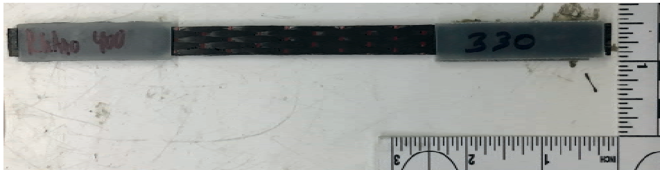
Figure 1.2 – Representative test specimen prior testing Scale in inches.
